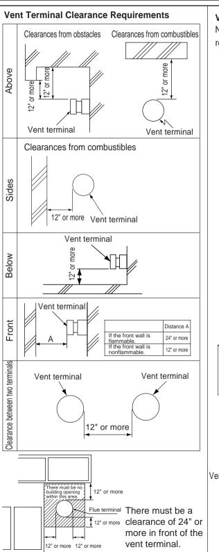
This restriction will not be applied to an area where an effective shield makes a clearance of 24" or more in front of the exhaust outlet.
