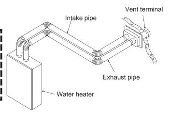
Connect the vent pipe to the vent terminal as follows:
