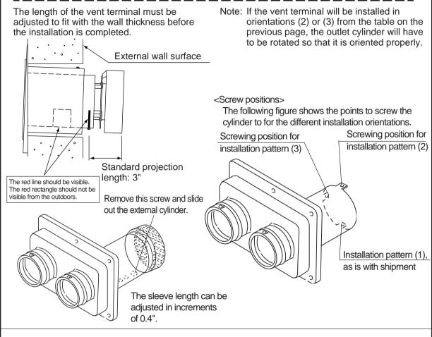
4) Attach vent terminal to the wall flange.
