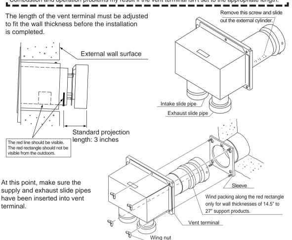
5) Extend the supply and exhaust slide pipes to connect the vent terminal to the water heater.
