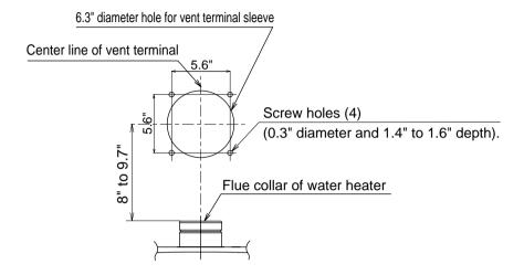
2) Adjust the sleeve length to fit the wall thickness. Install the sleeve with the symbol on the top side.
