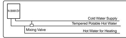
For Space Heating Purposes: If the system requires water for space heating at a higher temperature than for other uses, means such as a mixing valve shall be provided to temper the water for the other uses to help prevent scalding.
