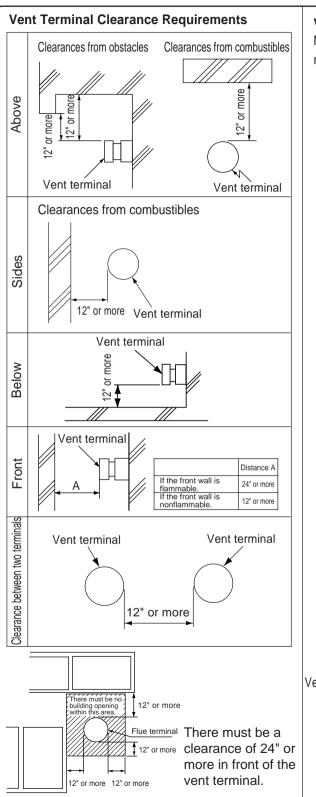
This restriction will not be applied to an area where an effective shield makes a clearance of 24" or more in front of the exhaust outlet.
