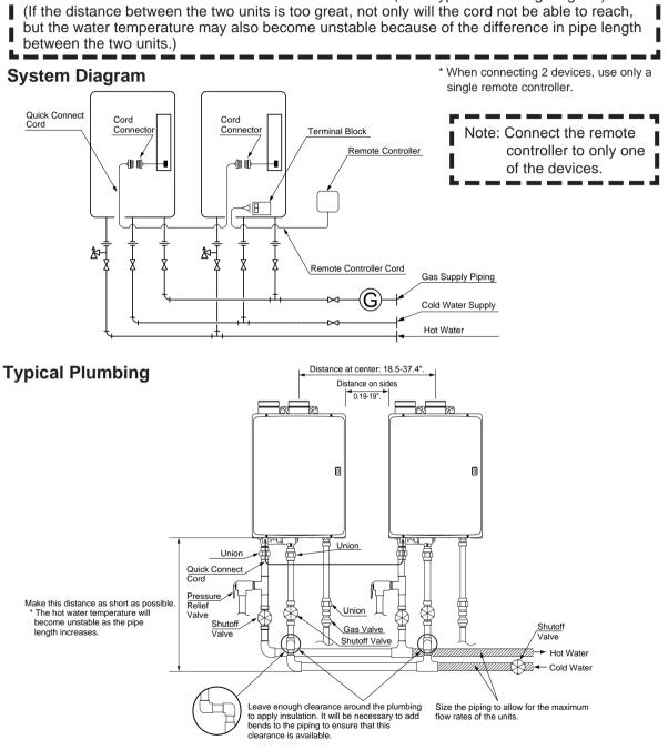
Insulate the hot water piping to prevent heat loss. Insulate and apply heating materials to the cold water supply piping to prevent heat loss and freezing of pipes when exposed to excessively cold temperatures.
