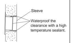
2) Attach the wall flange to the sleeve.
