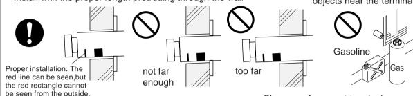
Avoid installing the terminal where obstacles will block it
